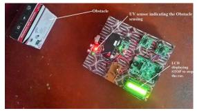
Fig: 6. Working of the Car When an Obstacle is Obstructed
