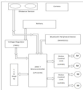
Fig: 1. Block Diagram ARM Based Remote Control Car
