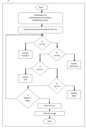
Fig: 5. Flowchart for the interfacing of smart phone with the RC car unit
